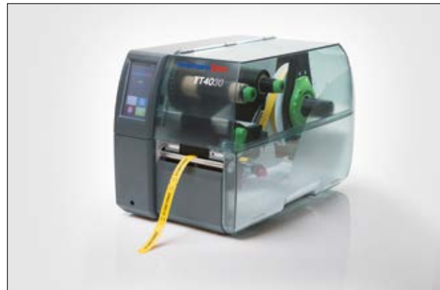
TT4030 thermal transfer printer for high volumes.
