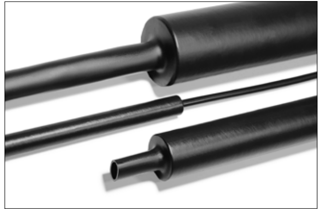
Medium wall tubing MA47 with shrink ratio 4:1 and adhesive liner.
