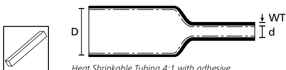
Heat Shrinkable Tubing 4:1 with adhesive
